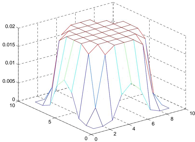
`h = fspecial('gaussian', hsize, sigma)` returns a rotationally symmetric Gaussian lowpass filter of size `hsize` with standard deviation `sigma` (positive). `hsize` can be a vector specifying the number of rows and columns in `h`, or it can be a scalar, in which case `h` is a square matrix. The default value for `hsize` is [3 3]; the default value for `sigma` is 0.5.
