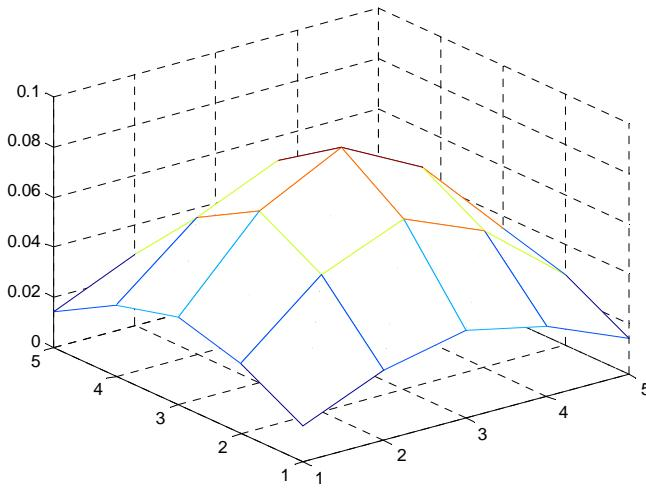
`h = fspecial('laplacian', alpha)` returns a 3-by-3 filter approximating the shape of the two-dimensional Laplacian operator. The parameter alpha controls the shape of the Laplacian and must be in the range 0.0 to 1.0. The default value for alpha is 0.2.
